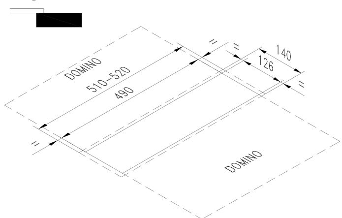
Flush mounting of the built-in units:
