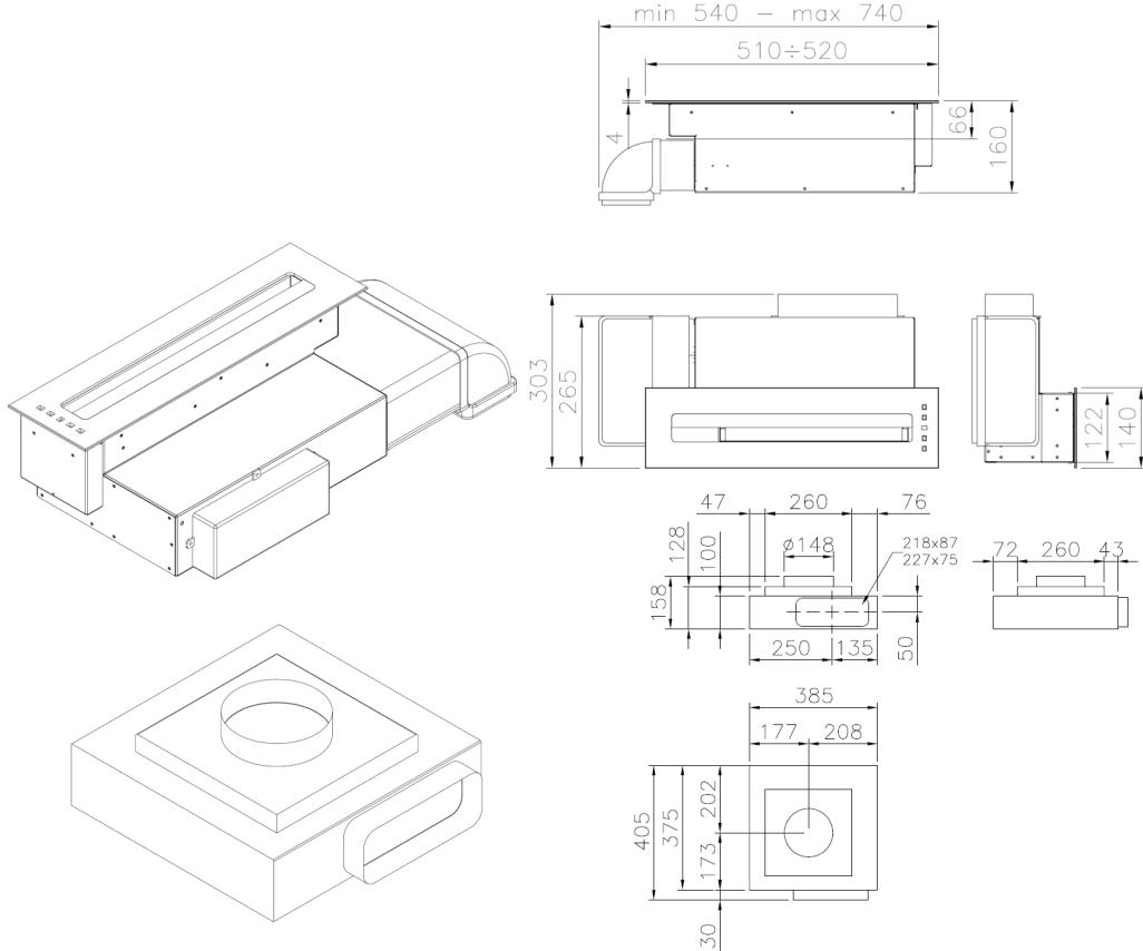
For the dimensions of the hole, see drawing here below (ATTENTION: one hole hood - domino)
